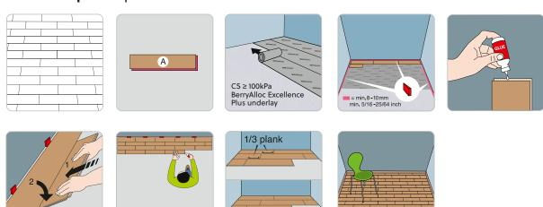
If you choose the shipdeck pattern, you only need the A-planks. Put a first plank in the corner of the room with groove side pointing towards the direction of the installation. Apply glue to the short side of every plank before you install it. Make sure the joints of the planks are staggered 1/3 of their length.
